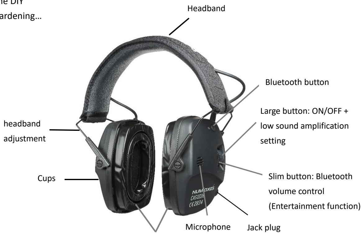
The headband and the cushions are the parts of the headset which are in touch with the user. They are composed of ABS, PU and silicone. Also, the headband force is not adjustable. The cushions composed of silicone are replaceable.
