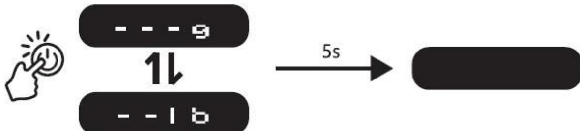
To change the unit of measurement, press the touch-sensitive on/off button lightly. The screen will automatically turn off after 5 seconds of inactivity.
