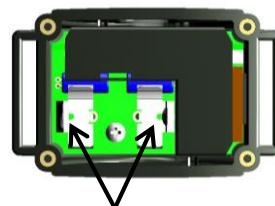
Reset: connect the 2 supports of the battery
