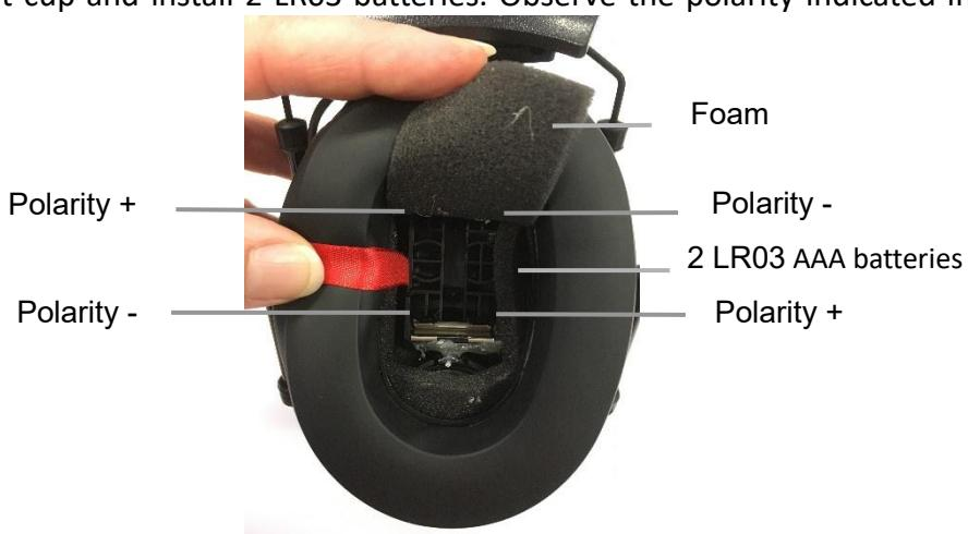
Whenever batteries are low, the red led (that lies on the cup) intensity fades. The more your batteries are getting low, the more the red light is going to fade. Whenever batteries are low, the headset does not turn and the low natural sounds are not anymore amplified. Then you need to replace the batteries. Please follow the previous section's procedure.
