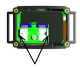
Reset: connect the 2 battery supports
