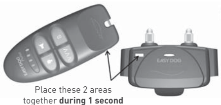
Diagram 6 Activate/Deactivate a receiver collar with an EASY DOG SOFT or EASY DOG PULSE remote control
